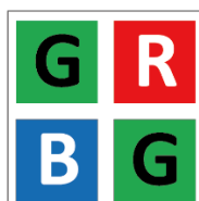
Figure 11-7 Bayer GR Pixel Pattern
