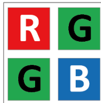
Figure 11-10 Bayer RG Pixel Pattern
