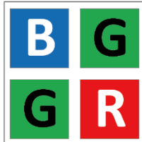
Figure 11-9 Bayer BG Pixel Pattern
