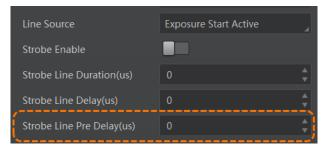
Figure 9-33 Set Strobe Pre Line Delay
