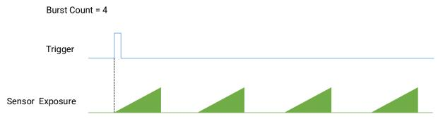
Figure 9-11 Sequence Diagram of Acquisition Burst Frame Count
