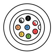
Figure 4-6 8-Pin M12 A-Code Control Interface
