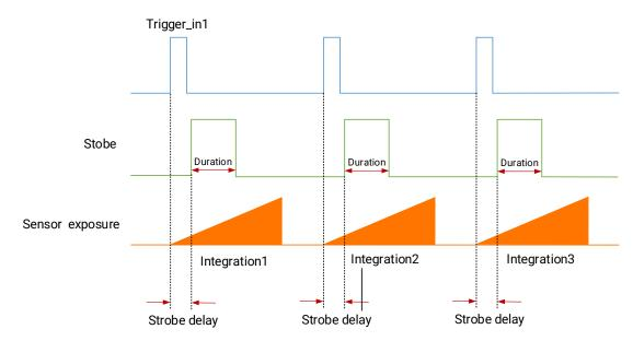
Figure 9-32 Sequence Diagram of Strobe Line Delay
