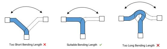
Figure 6-4 Suitable Bending Length
