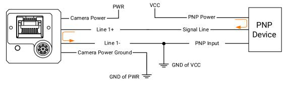
Figure 8-11 Output Signal Connects to PNP Device
