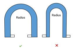
Figure 6-5 Sufficient Bending Radius
