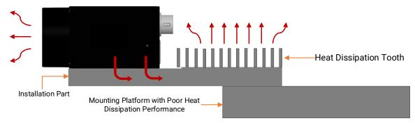
Figure 5-5 Add Heat Dissipation Tooth
