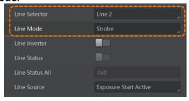
Figure 13-25 Select Line 2 as Output Signal
