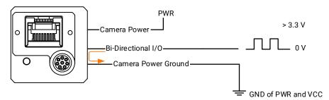
Figure 8-16 Input Signal Connects to Switch
