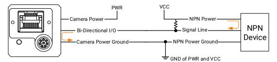
Figure 8-18 Output Signal Connects to NPN Device
