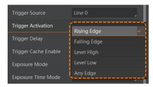
Figure 9-18 Set Trigger Activation
