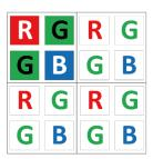
Figure 12-12Horizontal/Vertical Binning 2 × 2 (Color Device as an Example)
