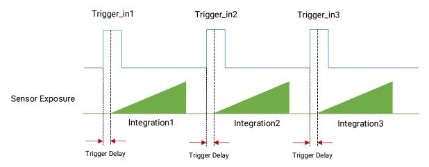
Figure 9-13 Sequence Diagram of Trigger Delay
