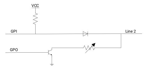
Figure 8-5 Internal Circuit of Bi-Directional Signal
