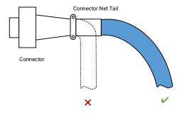
**Figure 6-6 Assemble Connector**
