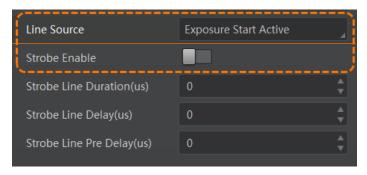
Figure 9-25 Enable Strobe Signal
