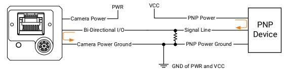
Figure 8-14 Input Signal Connects to PNP Device
