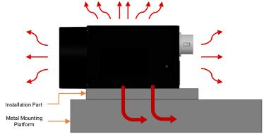
Figure 5-3 Heat Dissipation via Installation Part
