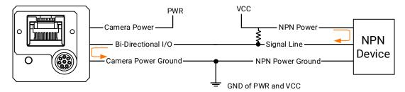
Figure 8-15 Input Signal Connects to NPN Device
