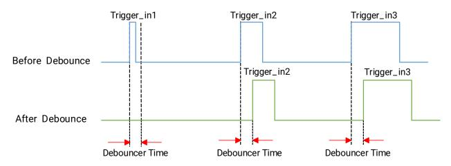
Figure 9-21 Sequence Diagram of Trigger Debouncer
