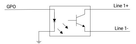
Figure 8-3 Internal Circuit of Output Signal
