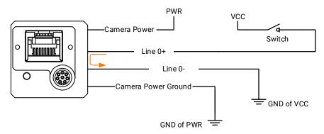
Figure 8-10 Input Signal Connects to Switch
