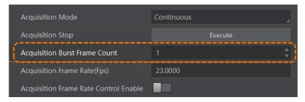
Figure 9-10 Set Acquisition Burst Frame Count
