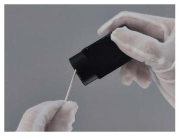
Figure 2-2 Contact Cleaning
