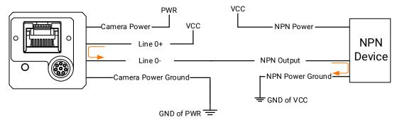
Figure 8-9 Input Signal Connects to NPN Device
