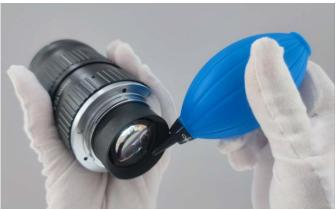
Figure 2-1 Cleaning by Rubber Dust Air Blower
