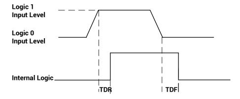
Figure 8-2 Input Logic Level
