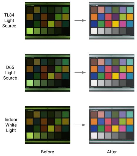
Figure 13-17 Automatic Color Correction Example
