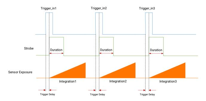
Figure 9-30 Sequence Diagram of Strobe Line Duration
