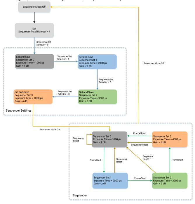
Figure 12-27 Principle of Sequencer
