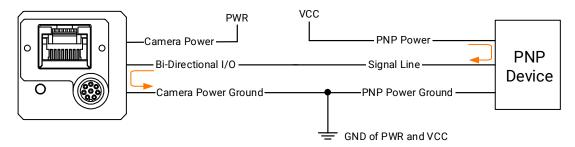
Figure 8-17 Output Signal Connects to PNP Device
