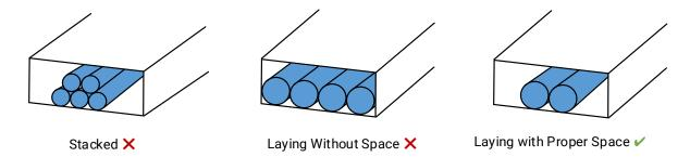
Figure 6-1 Cable Laying
