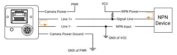
Figure 8-13 Output Signal Connects to NPN Device
