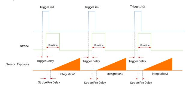
Figure 9-34 Sequence Diagram of Strobe Pre Line Delay
