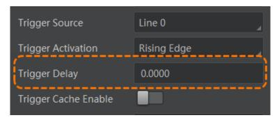
Figure 9-12 Set Trigger Delay
