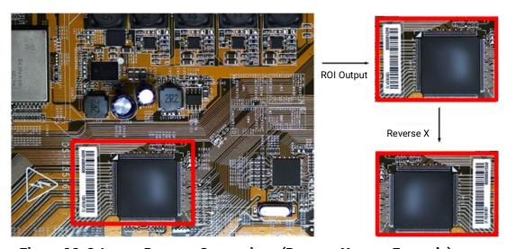
Figure 12-3 Image Reverse Comparison (Reverse X as an Example)
