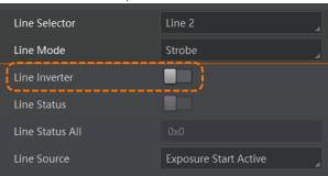
Figure 9-24 Enable Line Inverter
