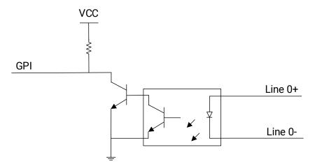
Figure 8-1 Internal Circuit of Input Signal
