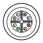
Figure 4-5 8-Pin M12 X-Code Connector
