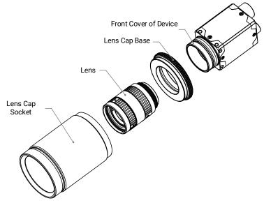
Figure 7-4 Install Lens and Lens Cap
