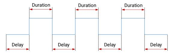
Figure 9-27 Sequence Diagram of Timer Active
