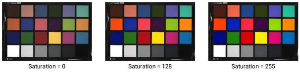
Figure 13-12 Saturation Example
