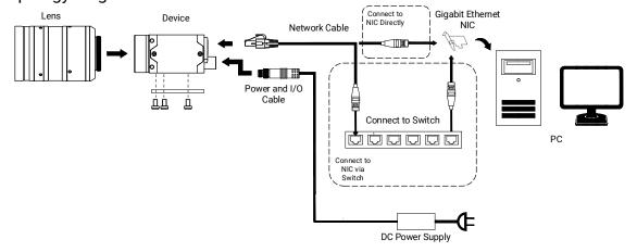
Figure 7-2 Topology Diagram of Device with BASE Version
