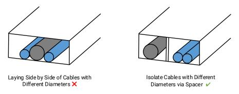
Figure 6-2 Isolated via Spacer
